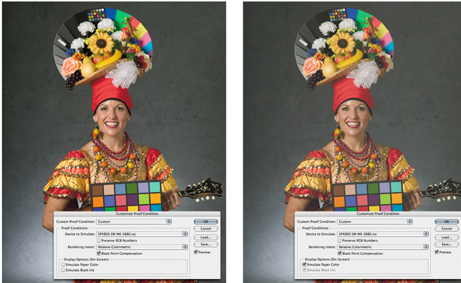
Soft proofing with Simulate Paper Color and Simulate Black Ink deselected (left) and selected (right)
